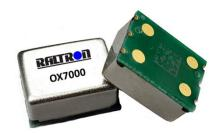
The OX7000 Series covers a frequency range from 5.000 MHz to 40.000 MHZ with a power supply voltage of 3.3 V at 150 mA steady state. The OX7000 Series OCXO combines ultra-small size with ultra-reliable frequency stability of +/-10 ppb.
