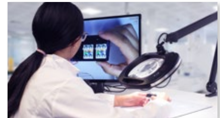
Inspect through a Monitor & Magnifying Lens
