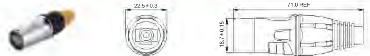
Metal Square Receptacle YT-RJ45-JSX-16-001
