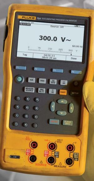
Loop calibrators are essential tools for working with 4–20 mA current loops. Fluke loop calibrators provide mA sourcing, simulation and measurement readouts in both mA and % of span along with a 24 V loop supply, simple operation and accuracy you can count on. Our HART-enabled loop calibrators help you get the most out of your smart transmitter calibrations, adding useful configuration capabilities and giving you more access and information on the HART devices you're testing.
