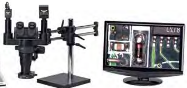
TKEZ-850-LV2 Shown with Optional Dual Trinocular Video Splitter and both HD 1080p and USB2.0 Inspection Packages
