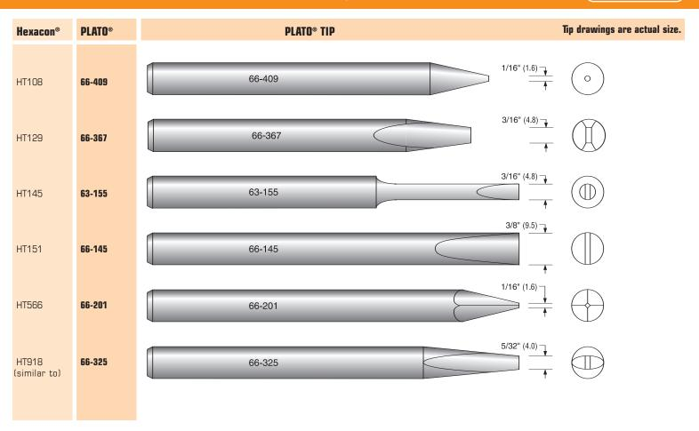
All points are 1/16" (1.6) thick unless otherwise noted. ( ) = mm Tip samples are available. Custom tip designs on request. All dimensions are shown before tinning and are subject to manufacturing tolerances.
