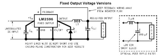
$C_{\text{IN}}$  = 470  $\mu\text{F},$  50V,  $C_{\text{OUT}}$  = 220  $\mu\text{F},$  25V (Aluminum Electrolytic Nichicon "PL Series"
