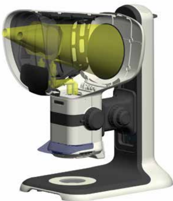
Twin (stereo) optical paths projected from the Dynascope® viewing head.
