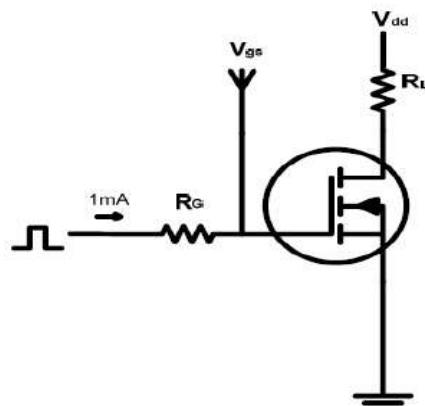
Switch Time Test Circuit:
