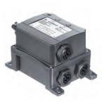
EnOcean 4-fold switching outputs in the IP68 surface housings for outdoor use feature four 230 V relays. They can be programmed for 30 push-button pairs. All electrical connections are pluggable.
